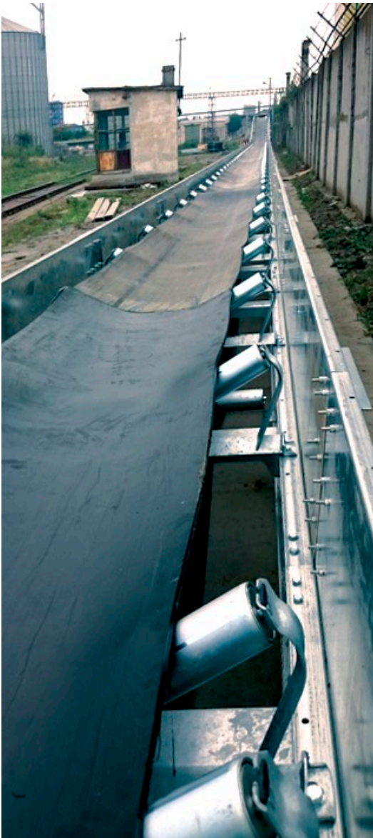
Anti-oil and anti-static belt mm 800.
