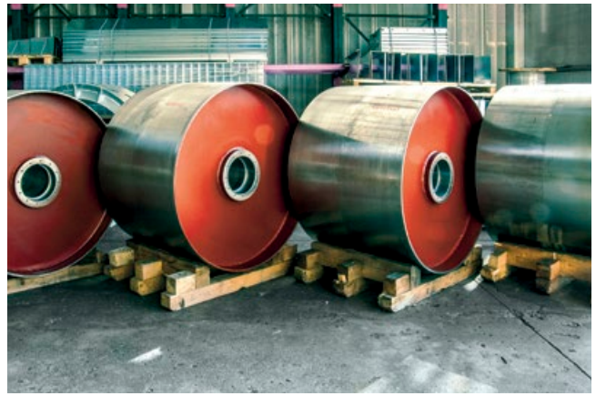
Pulley on head Ø mm 1250.
