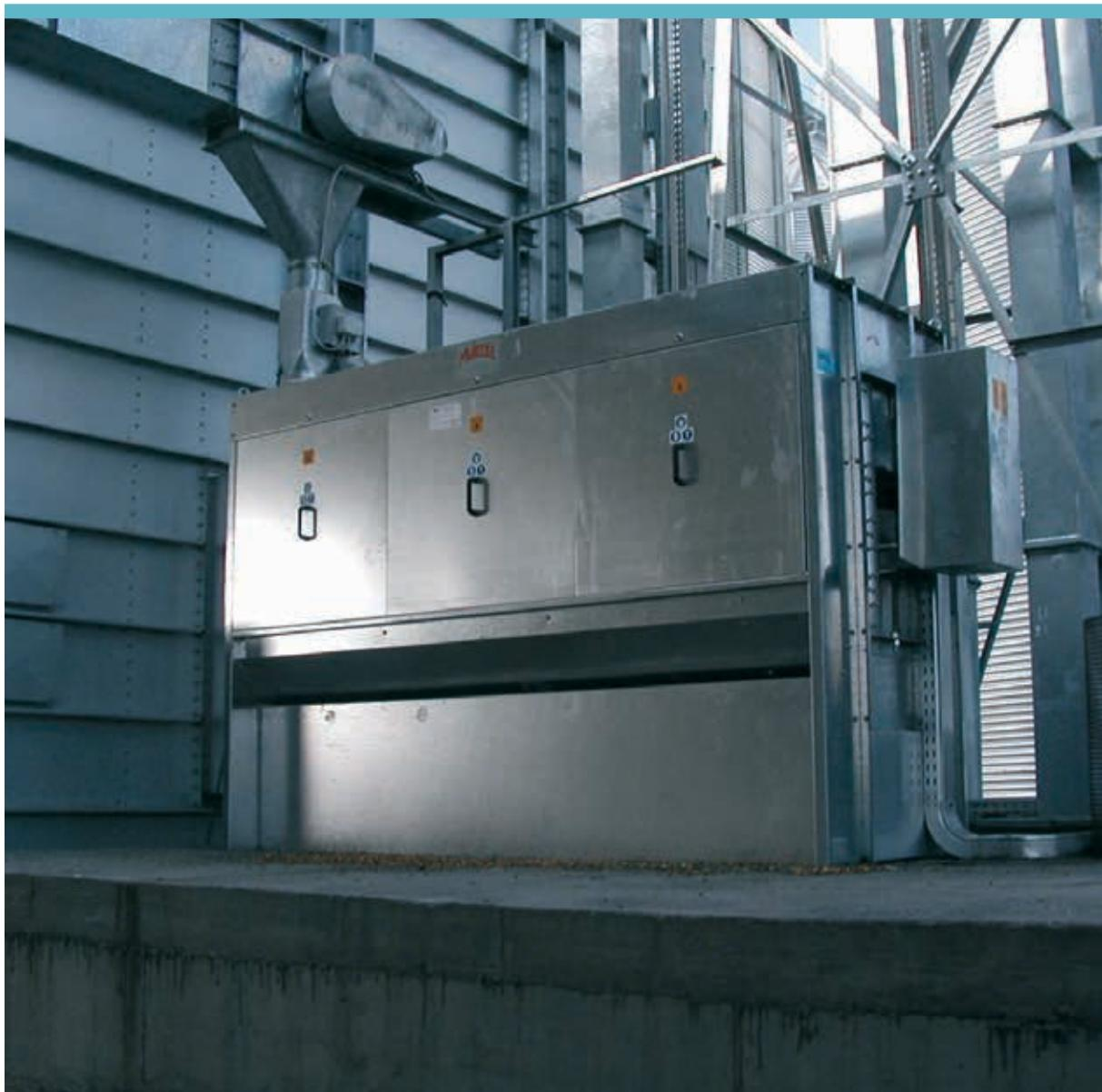
The PT drum cleaners are used in the pre-cleaning stage in order to separate the heaviest impurities from the cereals. They are built in conformity with the Machinery directive 2006/42/EC and for use in potentially explosive atmospheres are supplied according to the directive 94/9/EC.
